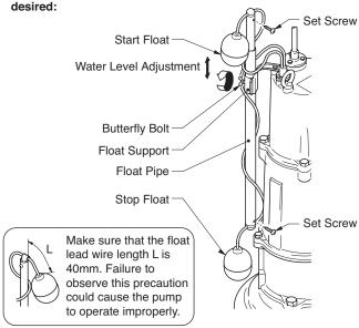
To change the operating water level on an automatic alternating model, perform the setting by referring to the diagram on the right.
